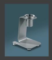
Flow Cup **Viscometers**
